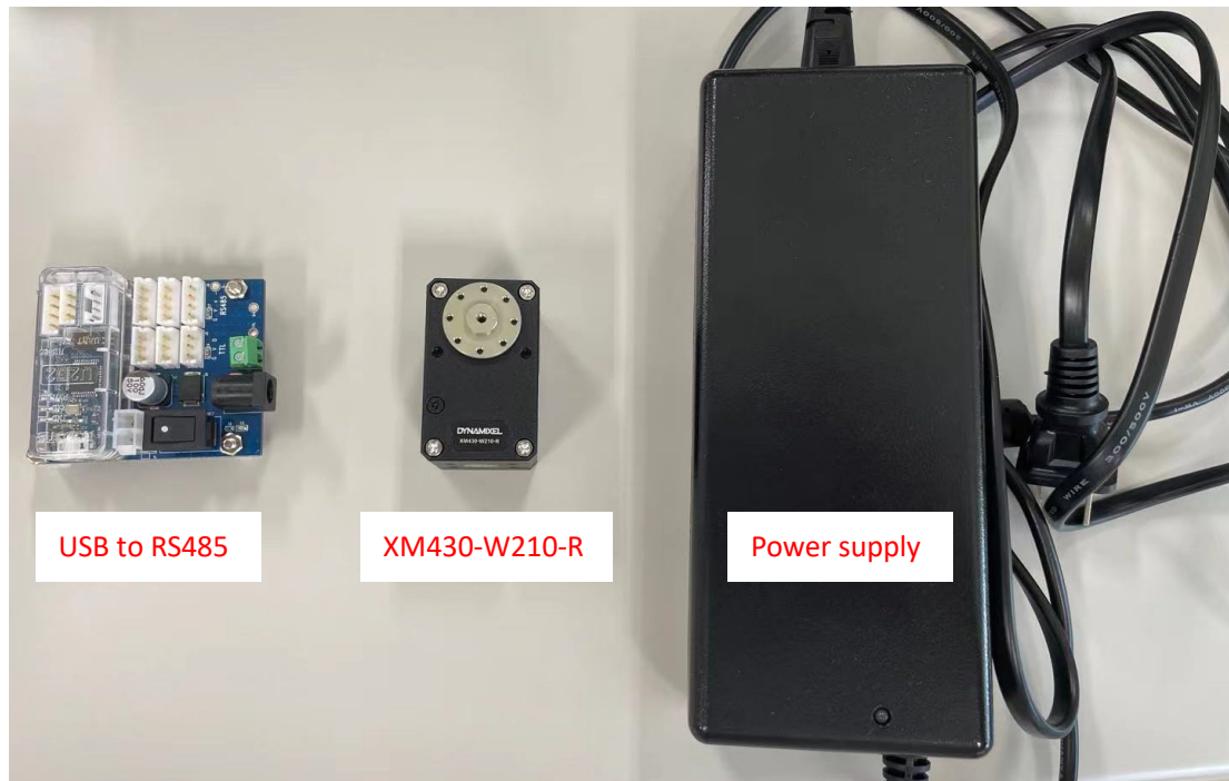
Figure 1: U2D2 Power Hub Board (left), XM430-W210-R (mid) and power supply (right).
