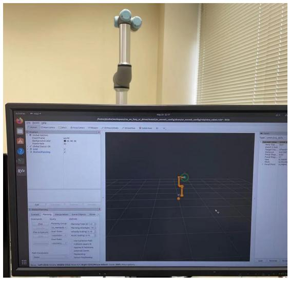
As shown in the above figure, now you can use the MoveIt Plugin in rviz2 to plan and execute trajectories with the robot.
