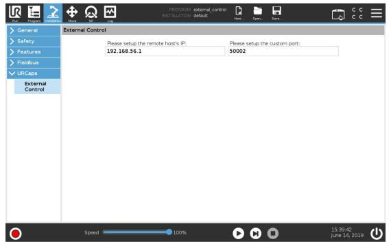
Step 4: Here you should setup the IP address of the external PC which will be running the
