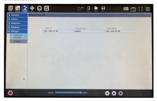
As shown in the above figure, configure the Host IP and Host name.
