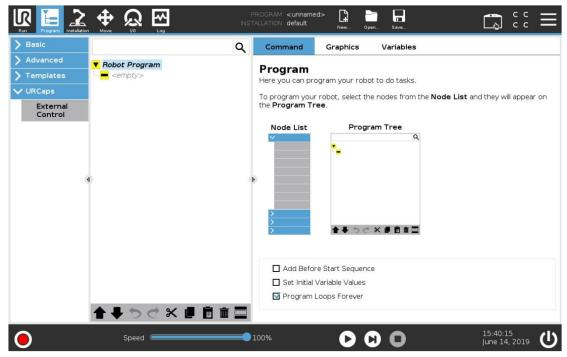
Step 5: To use the new URCaps, create a new program and insert the External Control program node into the program tree.
