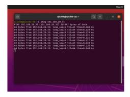
We can see the robot and the PC are successfully connected.
